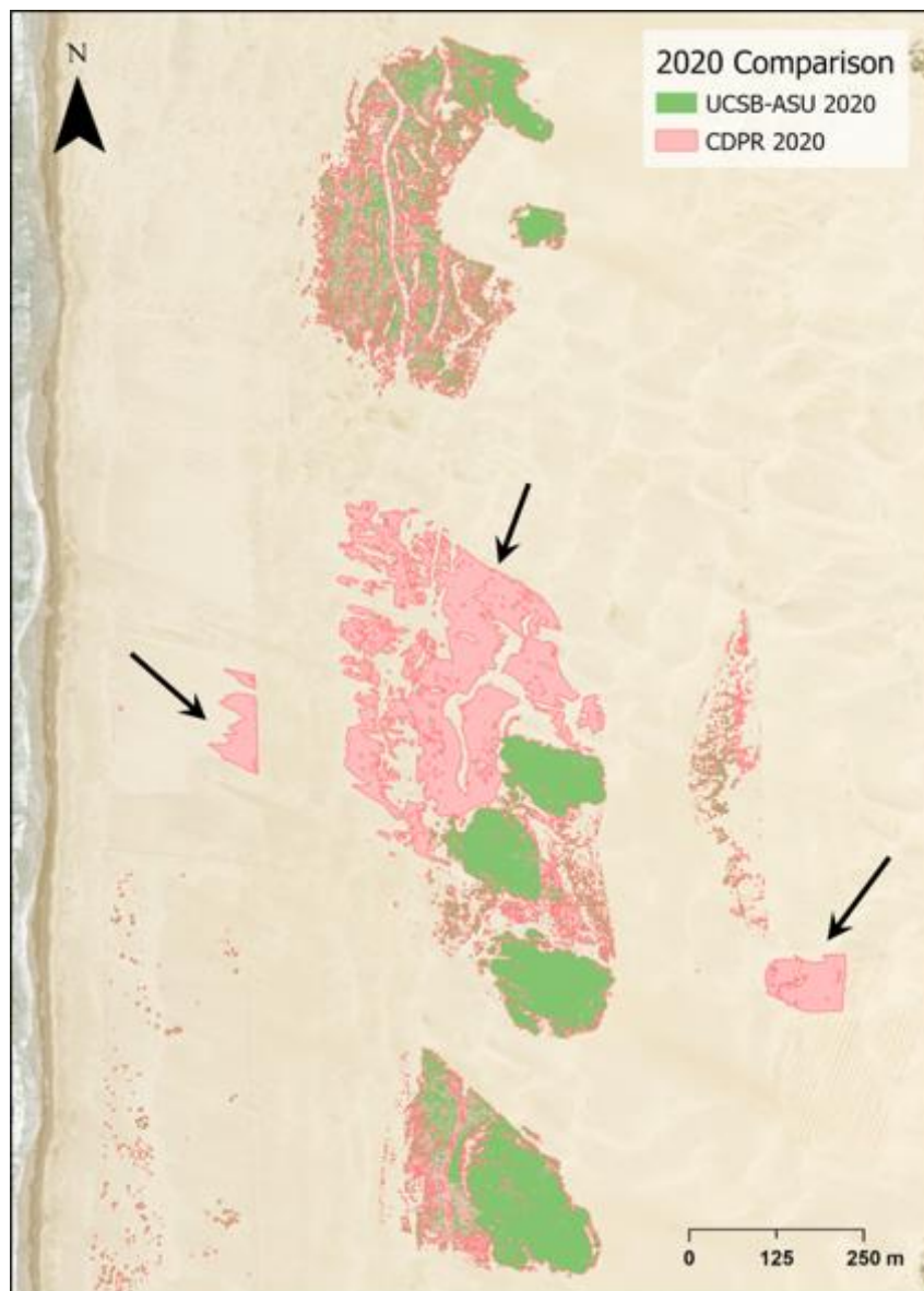
Figure 3. Vegetation cover analysis comparison between the CDPR report (pink) and the current report (green) for 2020 imagery. The arrows indicate areas where there is a straw treatment that was classified by CDPR as vegetation and by UCSB-ASU as non-vegetated area.
